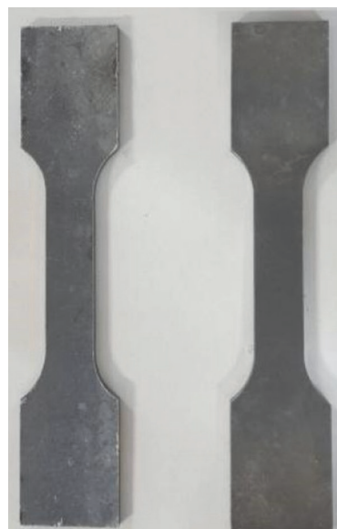
Figure 10. Specimen steel plate
